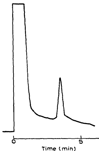
Fig. 3. Electron capture response to 25 pg of the hexakis-TMS ether of inokosterone. Operating conditions, as in Figs. 1 and 2; temperature, 275°.
